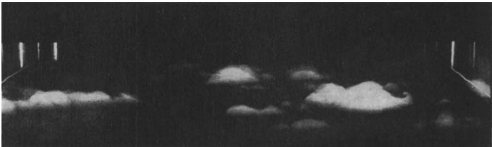
FIGURE 10. Oblique view from above of uppermost hummocks of the mixed layer at time t = 320 s in an experiment like E6 , showing the resemblance to cumulus-humilis clouds. Illumination is from both sides and is blocked below the simulated cumulus cloud base at a height of about 0.28 m. Converging lines on the left and right side walls are located at a height of 0.31 m, and are a distance 1.14 m apart.
